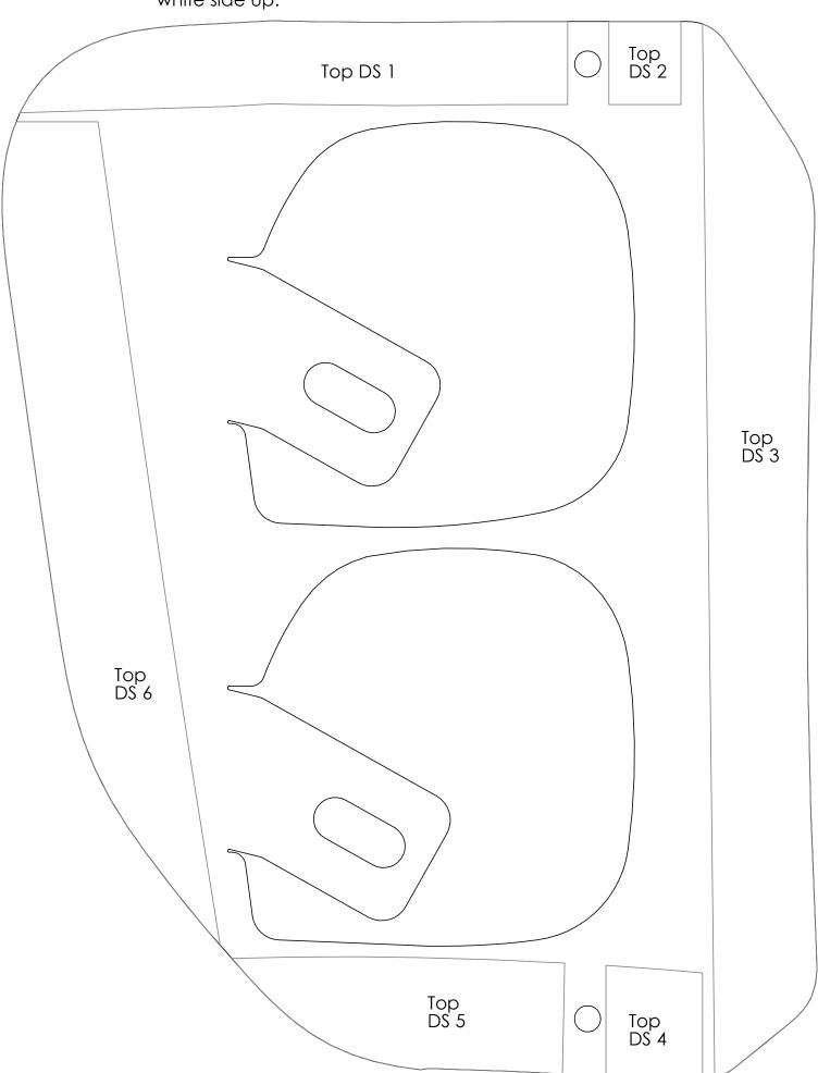
Passenger side bracket adhesive strip template - Cut out each of the six pieces and trace onto the rubber white side up.
