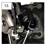
Interior Firewall Passthrough (Use lube when reinstalling)
